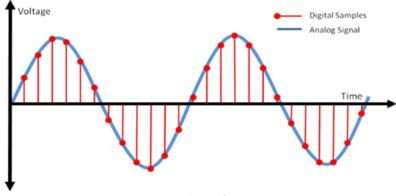
Figure1: Sampling of a sine wave
